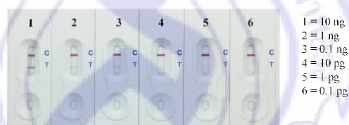
Figure 3 A series of the purified genomic DNA from S. aureus (10 ng to 0.1 pg) were used for the sensitivity test.
